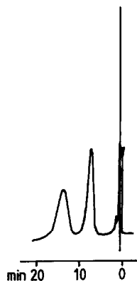
Fig. 4. Resolution of metoprolol enantiomers as oxazolidones. Column as in Fig. 3; mobile phase, phosphate buffer (pH 7.0; \mu = 0.02 ); flow-rate, 0.5 ml/min.
